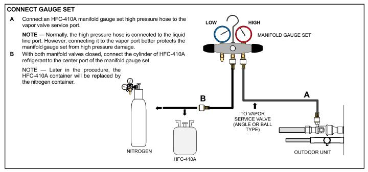
Figure 13. Manifold Gauge Set Connections for Leak Testing
